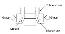
3. Put the boot-band as shown below, and tighten it.
